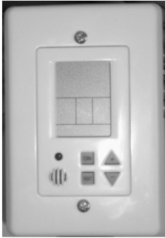
Figure 5 – Remote Thermostat Control
